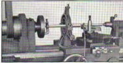
Using center rest to support long slender shaft while being machined
