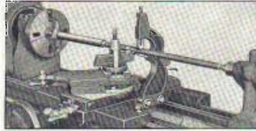
Cutting a screw thread on a long shaft with the aid of a follower rest.
