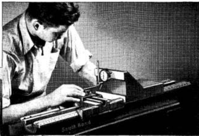
Fig. 6. Above—Testing the Saddle Cross Slide Dovetail for Squareness with V-Ways of the Lathe Bed
