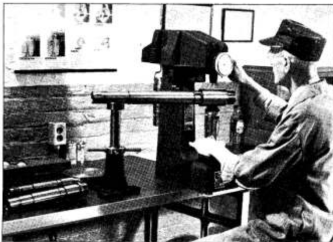
Fig. 4. Above—Testing the Hardness of a Carburized Headstock Spindle Bearing Surface
