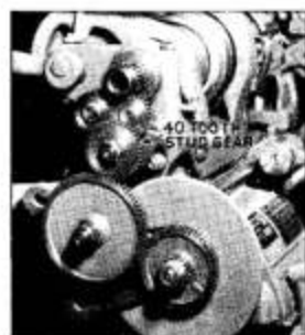
Lathe set up for cutting screw threads 4 to 7 per inch using 40-tooth stud gear
