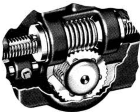
Fig. 18. (Above) Cut-away View Showing the Multiple Disc Friction Feed Clutch
