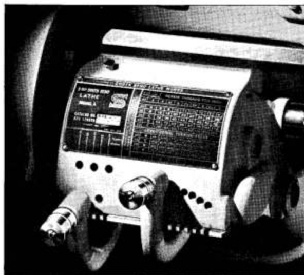
Quick Change Gear Box for Threads and Feeds Supplied as Standard Equipment on All Model A 9-inch Lathes
