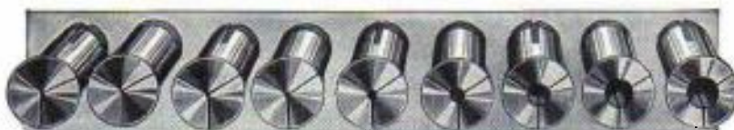
Fig. 69. Collets with Hole Sizes Ranging from \frac{1}{8} " up by Steps of 64ths of an Inch.
