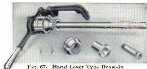
Fig. 67. Hand Lever Type Draw-in Collet Chuck Attachment.
