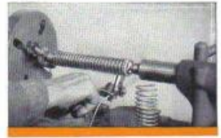
Fig. 40. Winding a Steel Spring in the Lathe. Attachment makes Springs from wire 0" to 1/8" in diam. Cat. No. 367. "Balun" $4.00
