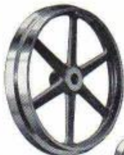
Fig. 124. Two-Step Pulleys for Countershaft and Motor. The large pulley is not grooved as the friction area is many times that of the motor pulley. Motor pulley is grooved.
