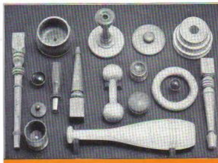
Fig. 122. Wood and Fibre Parts Machined in the 9-inch "Workshop" Lathe.
