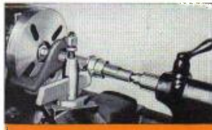
Fig. 49. Machining a Steel Sleeve Mounted on a Mandrel Between Centers in the Lathe.
