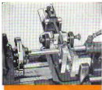
Fig. 109. Boring a Connecting Rod.
