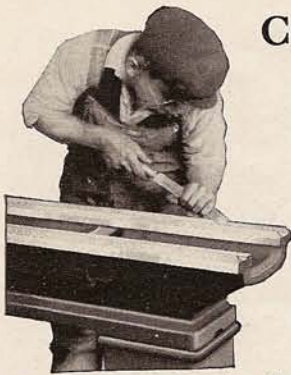
Fig. 108. Hand Scraping the Bearing Surfaces of the Lathe Bed
