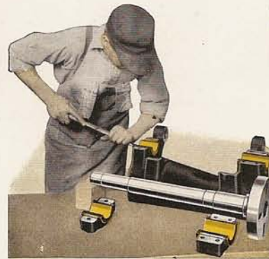
Fig. 20. Hand Scraping Phosphor Bronze Bearings for Headstock Spindle
