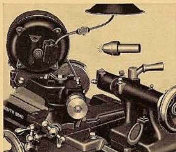
No. 14-B Electric Grinder Mounted on Compound Rest of Lathe.
