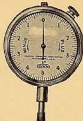
DIAL TEST INDICATOR Face of dial is graduated to record an error of one ten-thousandth of an inch.
