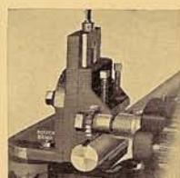
Milling a Standard Keyway
