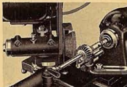
Sharpening a Reamer
