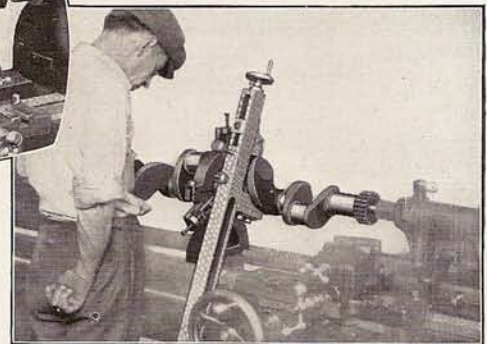
Fig. 15. Truing Main Bearings and Throw Bearings of Crankshaft with Weber Crank-pin Tool.
