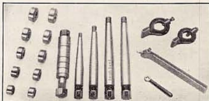
Fig. 11. Brake Drum Servicing Equip.
