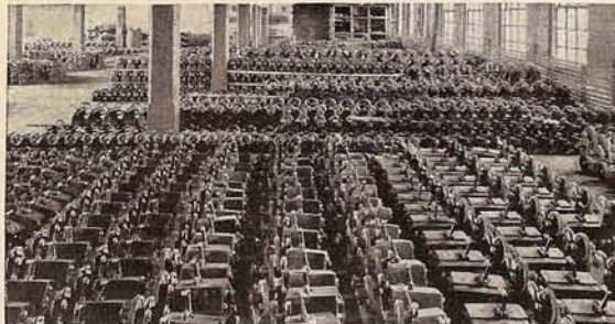
Headstocks, tailstocks, carriages, gear boxes, etc., carried in stock ready for assembly on the lathe
