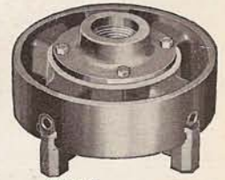
Fig. C Chuck with chuck-back attached, ready for use
