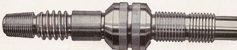
Fig. 27. Special Screw Showing Various Threads Cut on 9-inch "Workshop" Lathe.
