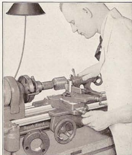
Fig. 22. Cutting a Screw Thread on the 9-inch "Workshop" Lathe.
