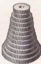
Fig. 21. Change Gears.
