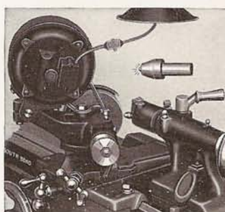
Electric Grinder with Diamond Holder and Diamond Dresser
