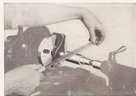
Fig. 32. Lathe is Practical for Filing and Polishing Bushings, Shafts, Parts, etc.
