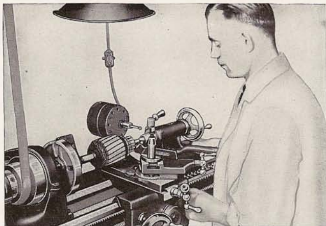
Fig. 47. Truing the Commutator of an Armature Mounted Between Centers in the Lathe before Undercutting the Mica Insulation.
