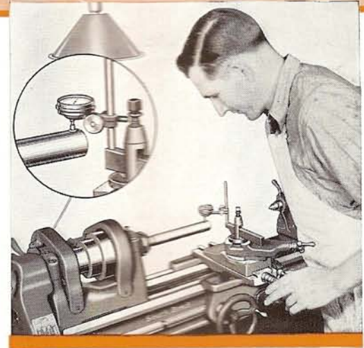
Fig. 24. Testing Alignment of Headstock Spindle with Lathe Bed, Using 6" Test Bar and Dial Indicator.
