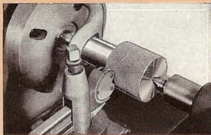
Fig. 41. Knurling a Large Handle Mounted Between Centers in the Lathe.
