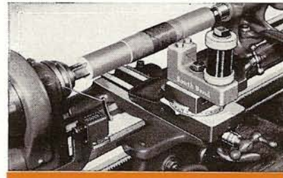
Fig. 50. Winding an Experimental Coil for a Radio. Note the Automatic Counter.
