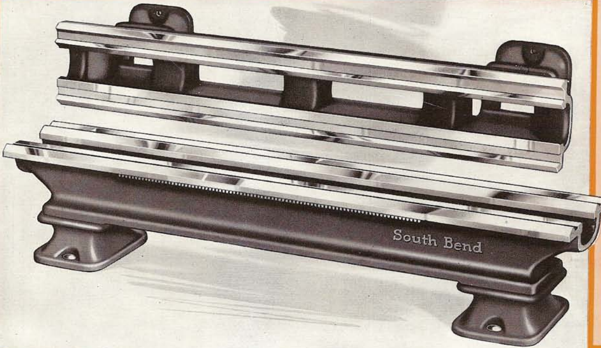
Fig. 20—Above. View of 9' x 3' Workshop Lathe Bed lying on its side to show top surfaces and box braces.
