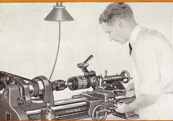
Fig. 102. Truing an Armature Commutator in the 9-inch "Workshop" South Bend Precision Lathe.
