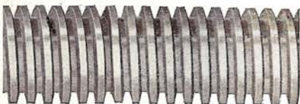
Precision Lead Screw used on 9-inch "Workshop" Lathe.
