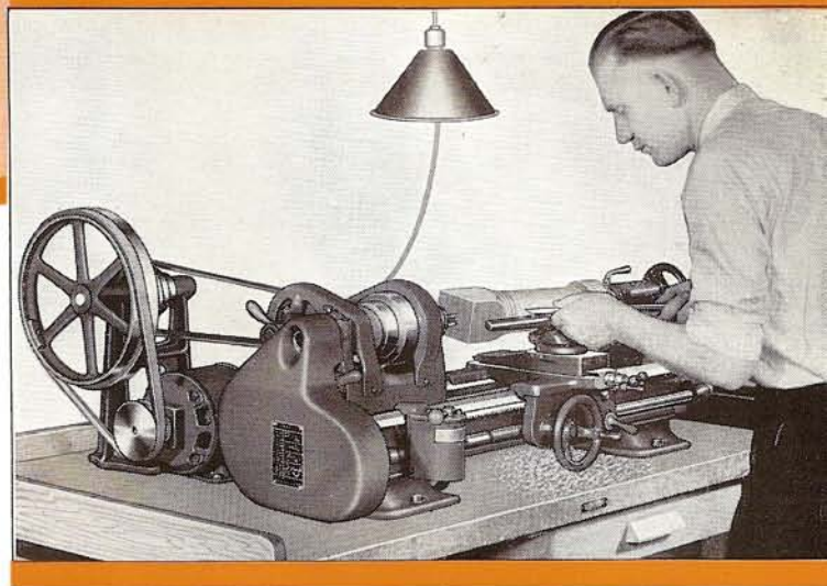
Fig. 120. 9-inch "Workshop" Lathe Equipped with 2-step Pulleys on Countershaft and Motor with Belt Arranged for Woodworking.
