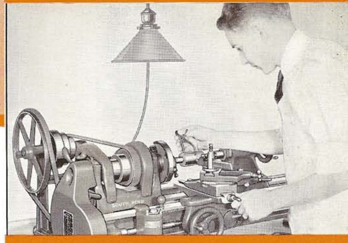
Fig. 111. Making a Replacement Bushing in the 9-inch "Workshop" South Bend Precision Lathe.
