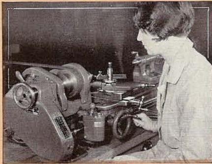
Fig. 36. 9" "Workshop" Lathe used for Production Work in the Manufacturing Plant.
