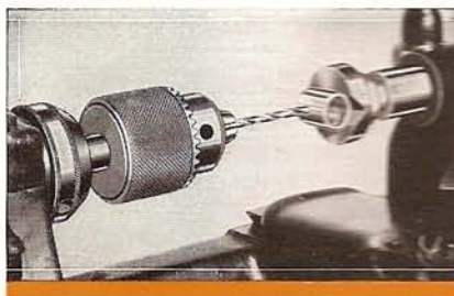
Fig. 42. Drilling a Bushing Supported in a Crotch Center.
