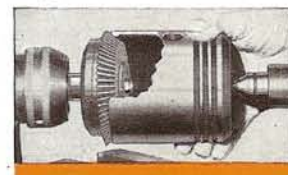
Fig. 107. Reaming the Skirt of a Piston Held on Piston Adapter.
