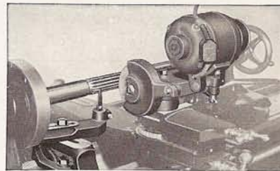
Sharpening a Straight Reamer
