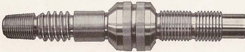
Special Screw Showing Various Types of Threads
