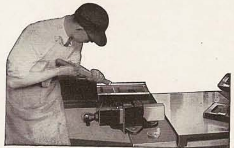
Hand Scraping Tailstock Base to Lathe Bed
