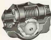
Fig. 17. Sectional view showing the multiple disc friction clutch.
