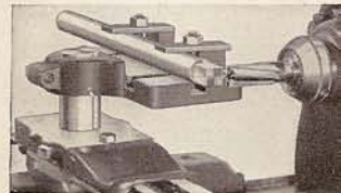
Fig. 78. Milling and Boring Table used to Square End of Shaft.
