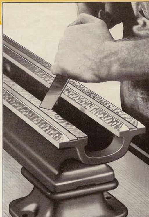
Fig. 8. Hand-Scraping the Bed of a 9-inch "Workshop" Lathe
