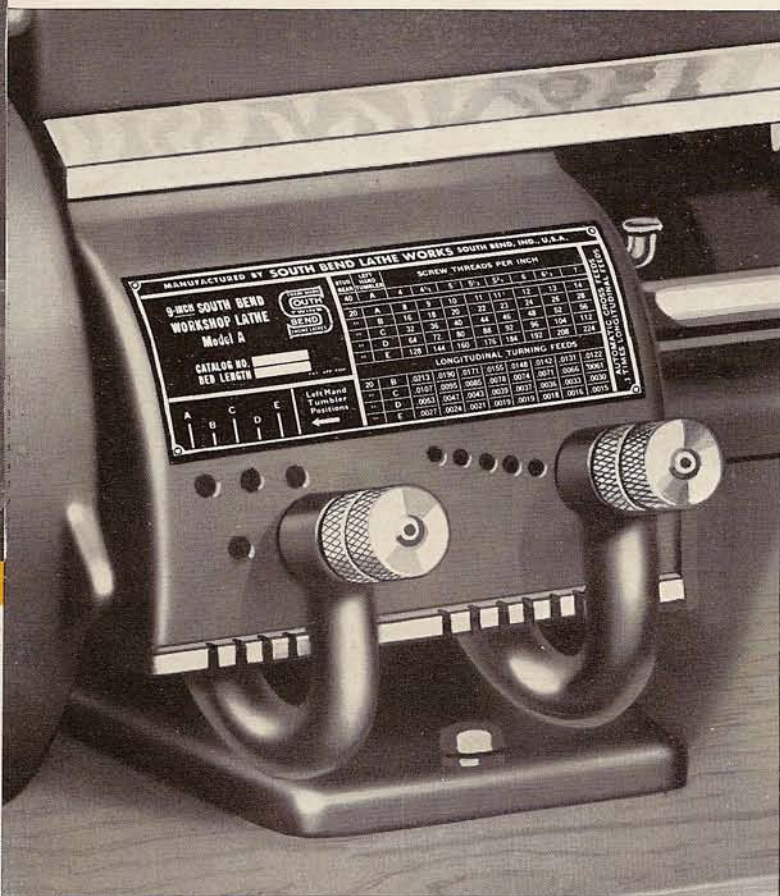
Fig. 45. Quick Change Gear Box for Threads and Feeds Supplied as Standard Equipment on All Model A 9-inch "Workshop" Lathes
