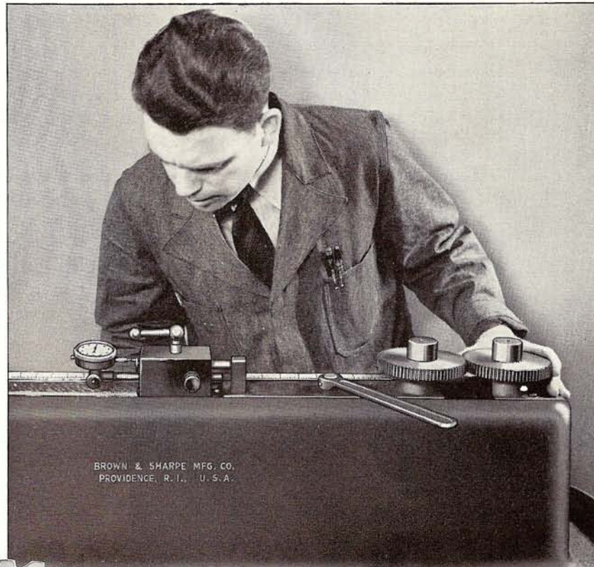
Fig. 25. Above. Precision Gear Testing Machine.
