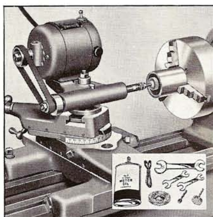
Fig. 71. High Speed Electric Grinder Mounted on Compound Rest of Lathe.
