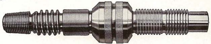
Fig. 37. Sample threaded piece showing variety of threads that can be cut on the 9-inch "Workshop" Lathe.
