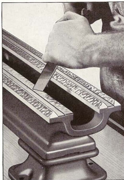
Fig. 18. Hand-Scraping the Bed of a 9-Inch "Workshop" Lathe.
