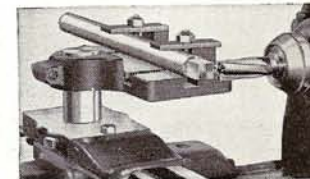
Fig. 61. Milling and Boring Table used to Square End of Shaft.
