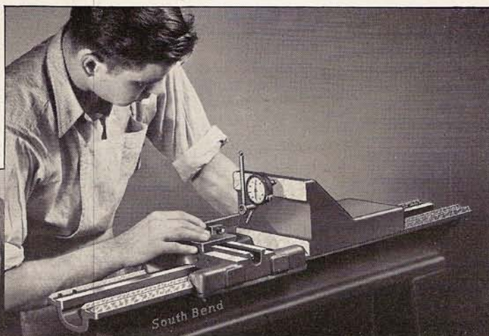
Fig. 6. Above—Testing the Saddle Cross Slide Dovetail for Squareness with V-Ways of the Lathe Bed
