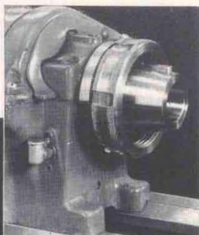
Right—Type L Long Taper Key Drive Spindle Nose.
