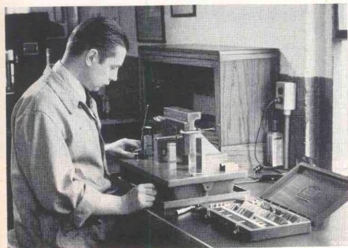
Fig. 4. Checking a Fixture with Precision Surface Plate and Lapped Gauge Blocks
