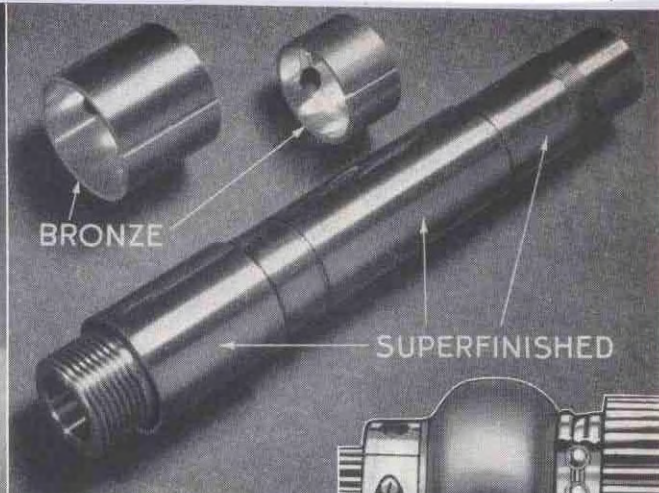
Fig. 17. Headstock Spindle and Bearings
