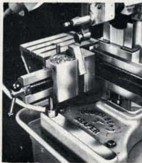
Bearing surface on base for adjustable table support
