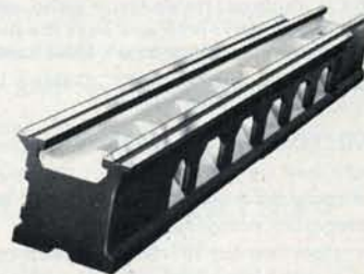
Three V-Way and one flat way all hardened and ground. Heavy side walls and cross bracing assure permanent precision alignment of headstock, tailstock and carriage. Inclined longitudinal bracing forms slide to discharge chips and coolant into slide-out chip pan.
