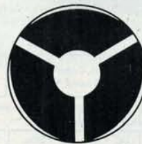
ROUND GROUND COLLETS In closing, force is exerted on edges of taper segment.
