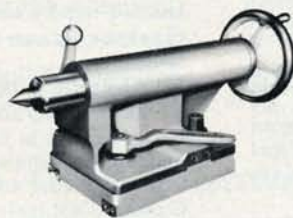
The tailstock design includes a barrel clamp that exerts upward pressure on the 2 1/2" spindle. This prevents misalignment—Spindle has tang slot and 6" of travel. Centers self ejecting. Two screws at front set over tailstock in either direction.
