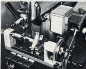
Machining flat surfaces on shaft with indexing head
