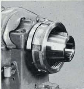
LOO Long taper key drive spindle. See page 36.
