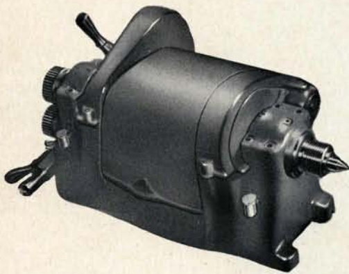
Headstock, cone pulley type with underneath belt drive.
