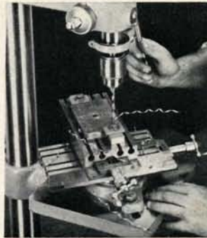
Precision drilling operation with use of a universal table for handling and clamping of work. See page 46.
