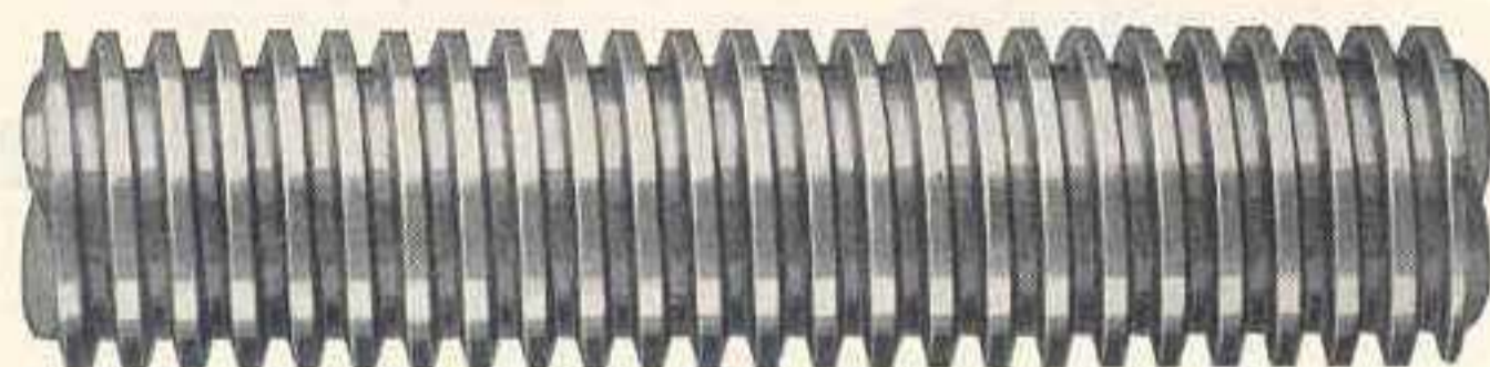
Fig. 46. Section of Lead Screw—Actual Size.
