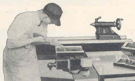
Fig. 36. The headstock, tailstock and saddle are hand scraped to a perfect bearing.
