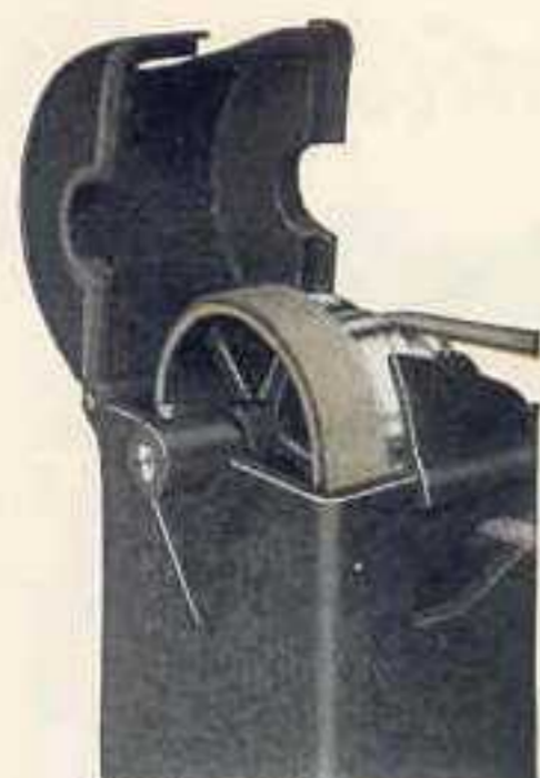
Cabinet Top Open to Show Drive Pulley.
