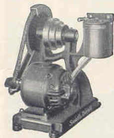
Self-Contained Motor Drive Unit, gear guard removed.
