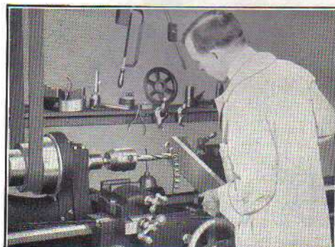
Using the Lathe as a Drill Press
