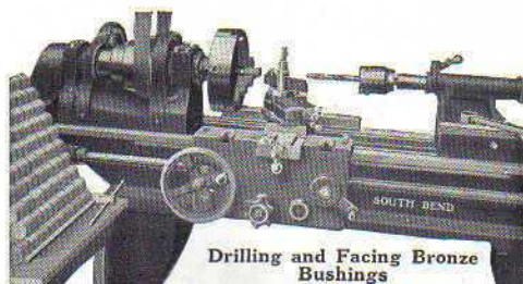
Using the Lathe as a Drill Press
