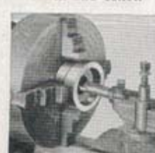
Boring a steel collar held in a 4-jaw Chuck.
