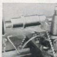
Making a steel bushing held on mandrel.
