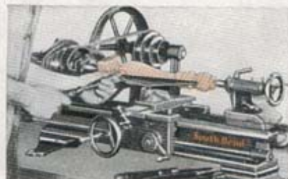
Turning a Large Diameter Ornamental Wood Column. For Hand Rests see page 11.
