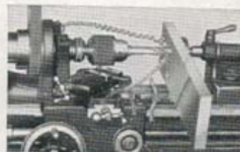
Drilling a steel plate held against the drill pad in the tailstock.
