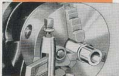
Making a Bronze Bushing from Bar Stock in the Lathe.
