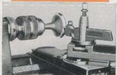
Refacing a 45° auto valve held in a Hollow Drill Chuck.
