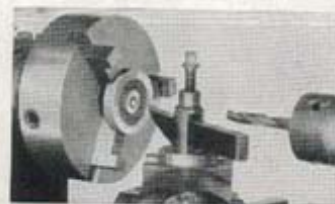
Centering a gear blank preliminary to drilling and boring.
