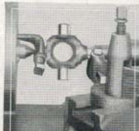
Turning a knuckle between centers in the lathe.
