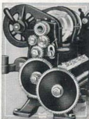
Screw thread gearing of 8-inch Junior Lathe.
