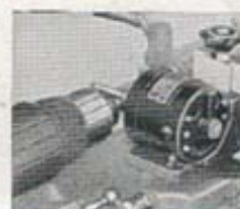
Undercutting Mica Insulation with mica undercutting attachment.
