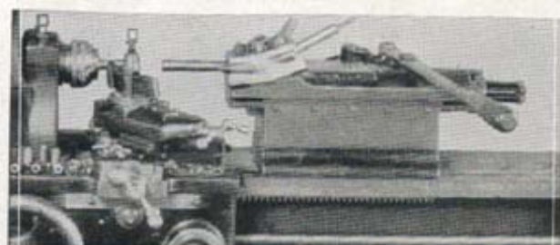
Manufacturing duplicate parts from bar stock using hand lever bed turret. Seven operations are performed at one setting.
