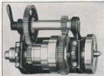
Back-Gear Headstock seen from above.
