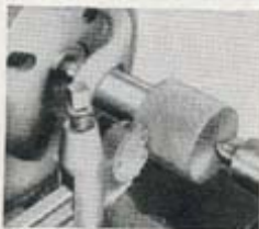
Knurling in the lathe.
