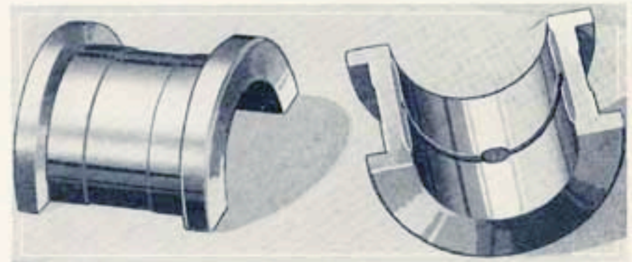
Fig. 11. Front Bearing for Headstock Spindle. Rear Bearing is similar to Front Bearing, but smaller in size and is not shown here because of lack of space.
