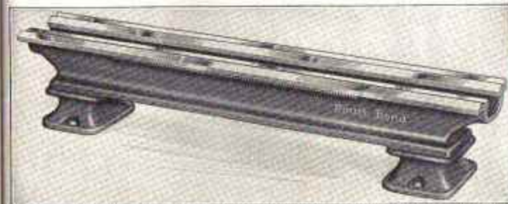
Fig. 21. View of 9'x3' "Workshop" Lathe Bed. Bed has 3 V-ways and 1 Flat Way
