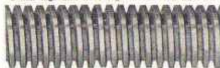
Fig. 22. Precision Leadscrew Used on 9-inch "Workshop" Lathe
