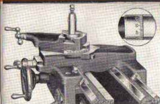
Fig. 20. Saddle and Compound Rest Used on the 9-inch "Workshop" Lathe with Close-up Showing Micrometer Graduated Collars on Compound Rest and Cross Feed Screws
