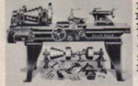
1 - 16" swing x 8' bed Slightly Used Quick Change Gear South Bend Back Geared Screw Cutting Lathe with double friction countershaft. In perfect condition, like new. Catalog No. 92-E, takes 58" between centers. Complete with regular Lathe equipment as illustrated under Lathe. Regular catalog price \$638.00, we are reducing this price \$223.00. The Bargain Price, f.o.b. South Bend, Ind., is ...
