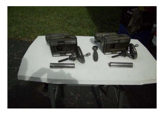
The newer TS spindle has a key that extends the entire length of the spindle. This may NOT be factory, as the pin that is supposed to hold the key to the spindle is not there, but there is a hole. Probably only gunk is holding the key in place.
