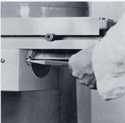
Fig. 20. Adjusting longitudinal feed gib.
