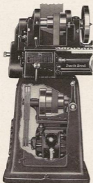
Fig. 33. Front View of Lathe with Underneath Belt Motor Drive Unit.
