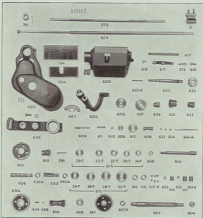
Fig. 8. Quick Change Gear Box Parts for Series "S" South Bend Quick Change Gear Lathes.
