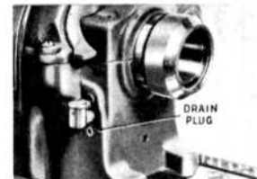
Drain and flush headstock every 3 months
