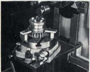
Machining clutch teeth with rotary indexing table.
