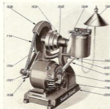
Self-Contained Motor Drive Unit with portion of Chain Guard cut away
