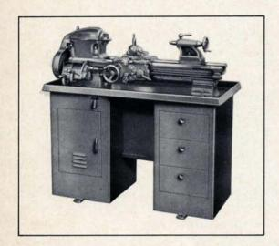
Cabinet type lathes are the same as the bench models except for underneath drive, spindle speeds and necessary alterations in the headstock. Cabinet has three drawers. Built-in chip pan forms the top of the cabinet.
