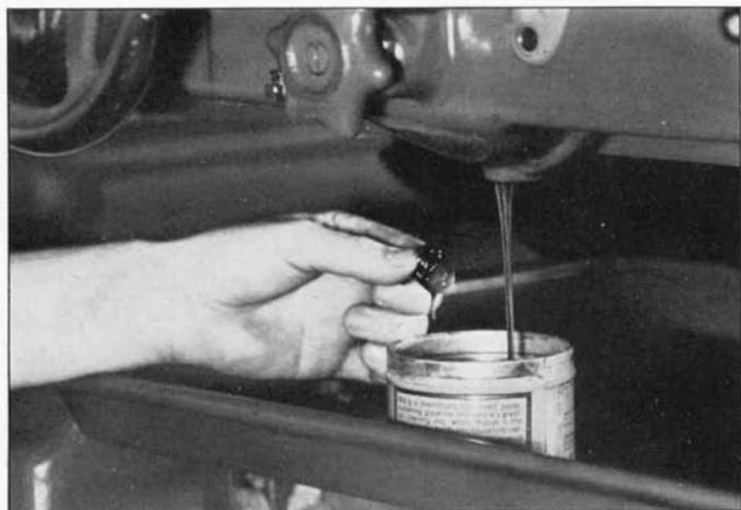
Fig. 7. The apron oil reservoir should be drained and flushed with kerosene occasionally.
