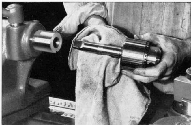
Fig. 15. Use a clean cloth to wipe the taper shank of a lathe center or drill chuck before mounting in spindle taper.
