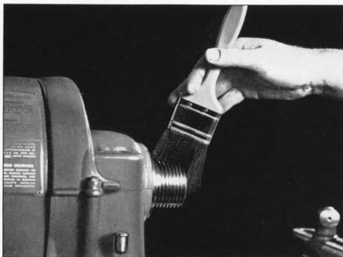
Fig. 10. The threads on the lathe spindle should be thoroughly cleaned and oiled before mounting a chuck or a face plate.
