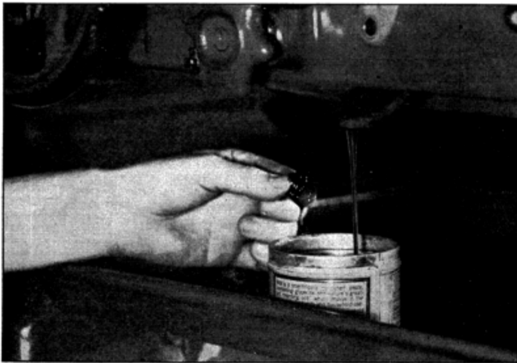
Fig. 15. The apron oil reservoir should be drained, flushed, and refilled every three months.
