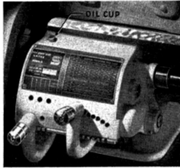
Fig. 12b. Gear box with single oil hole on top.
