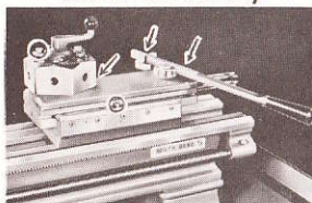
Oiling points on Handlever Bed Turret. TYPE "C" oil at all points. Oil Daily.
