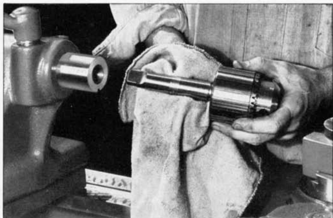
Fig. 15. Use a clean cloth to wipe the taper shank of a lathe center or drill chuck before mounting in spindle taper.
