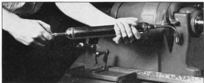
Fig. 8. Use a suction pump to drain the headstock oil reservoirs.
