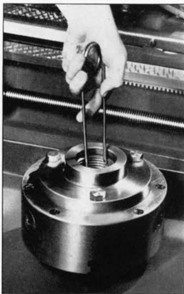
Fig. 12. The threads in the chuck-back should be carefully cleaned to remove all dirt and chips.
