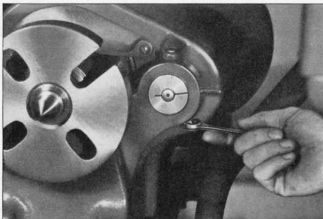
Fig. 16. Adjusting back-gear eccentric shaft tension bushing.
