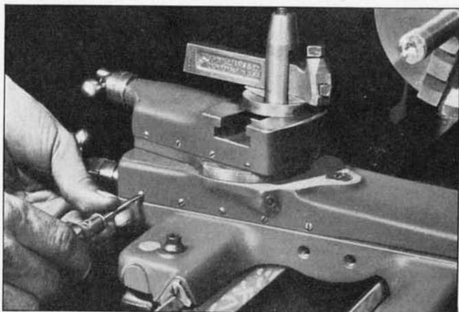
Fig. 24. Adjusting straight dovetail gib.
