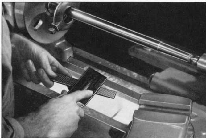
Fig. 37. Use a file card to clean chips out of files—never rap a file on the tailstock or other parts of lathe.
