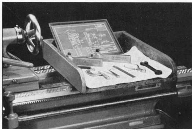
Fig. 36. A tool tray is convenient and eliminates the temptation to lay tools on the lathe bed.
