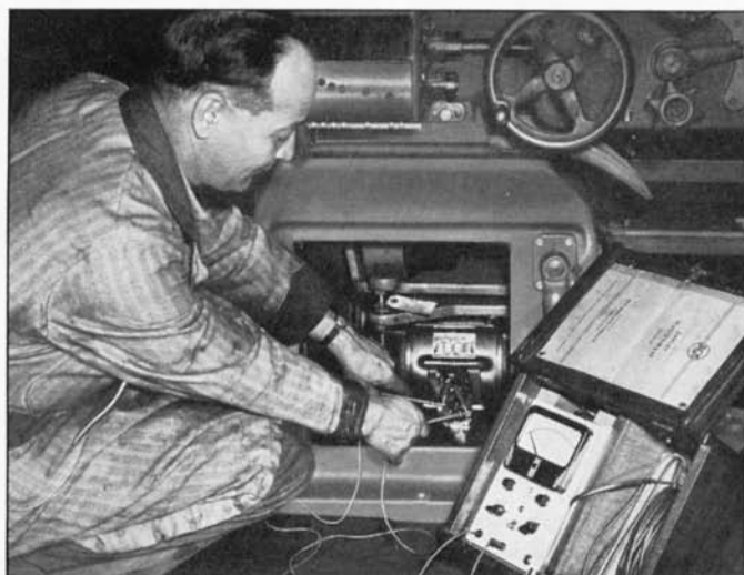
Fig. 2. Checking the line voltage at the motor.
