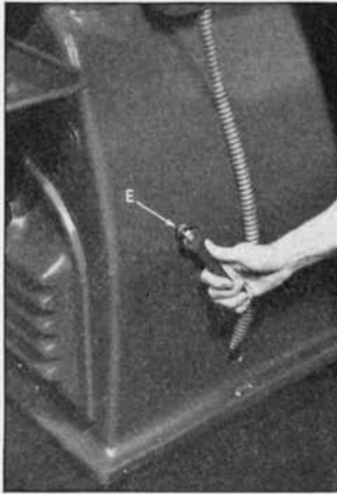
Fig. 6. If lathe is equipped with stop screw "E", it must be unscrewed before adjusting belts.
