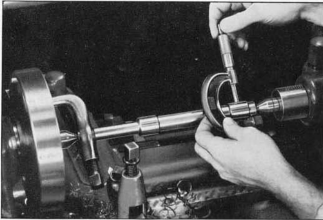
Fig. 31. Testing alignment of centers.
