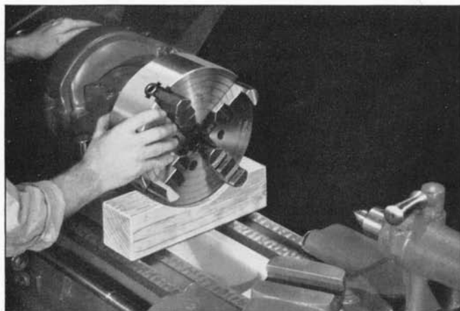
Fig. 35. Use a board to support heavy chucks when mounting or removing from lathe spindle—do not let chucks fall on lathe bed.
