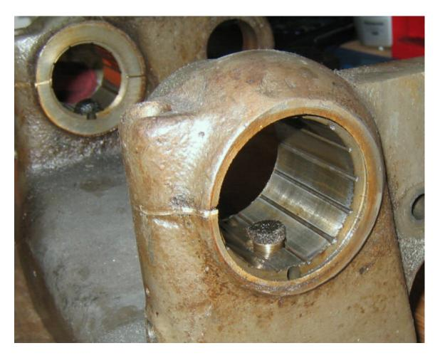
Before inserting the spindle, lubricate the inside of the spindle cone pulley with Teflon grease, and also make sure that all bearing surfaces of the spindle and bearings are coated with oil. Take care to line up the key for the backgear before assembly. This time you need to whack on the nose-end (threaded end) to get the back gear seated. Be **extremely** careful to protect the spindle nose from the hammer blows.
