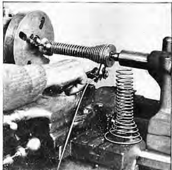
Fig. 643.—Winding a spiral spring on a special shaped arbor held between centers on the lathe.
