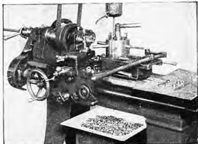
Fig. 611.—Screw cutting lathe fitted with a hand lever turret for machining small gear blanks.
