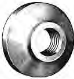
Fig. 504.—Semi-Machined Chuck Plate, threaded to fit the spindle nose of the lathe
