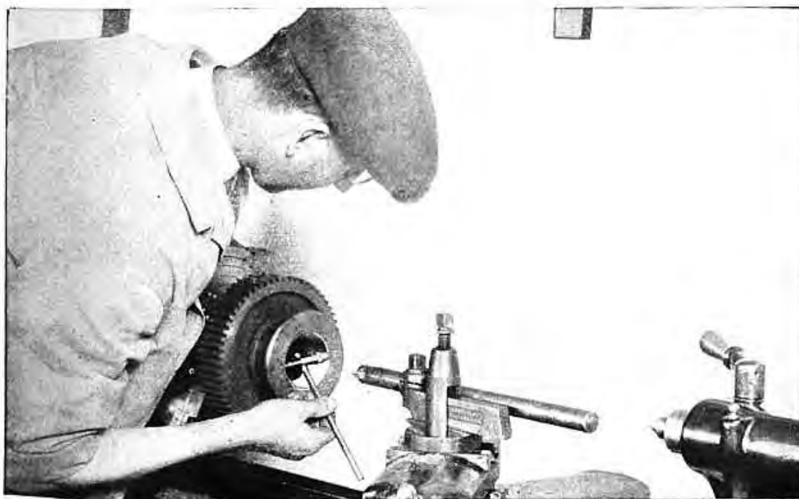
Fig. 440.—Using an Internal Micrometer Caliper Measuring the Diameter of a Machined Hole
