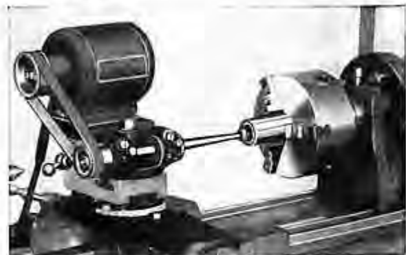
Grinding the inside of a steel bushing
