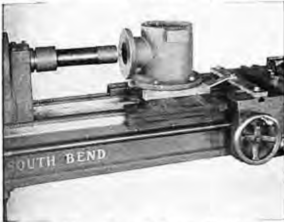
Fig. 640.—A cast iron T clamped to a special carriage on the bed of the lathe while being machined.
