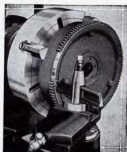
Fig. 633.—Machining Fly-wheel for New Ring Gear by Undercutting Worn Teeth with Parting Tool
