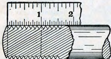
Fig. 557.—Measuring Screw Threads
