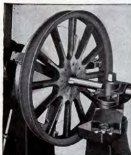
Fig. 631.—Boring a Wood Wheel, Mounted in Chuck, for New Hub
