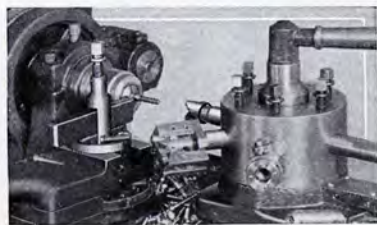
Fig. 608.—Using a Draw-in Chuck and Turret for Making Small Screws
