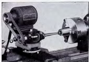
Grinding the inside of a Steel Bushing
