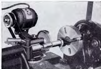
Grinding a Hardened Steel Bushing
