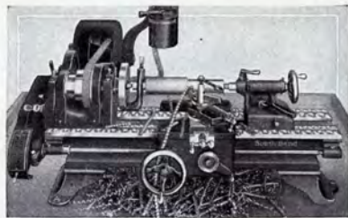
Taking a Chip on a Steel Shaft, in the 9-inch Horizontal Motor Drive Lathe
