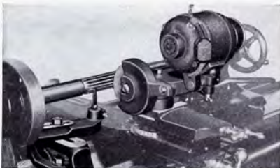
Grinding a Straight Reamer in the Lathe
