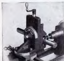
Fig. 589.—Milling a Woodruff Keyway
