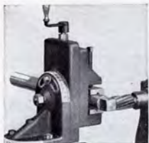
Fig. 588.—Squaring the End of a Shaft
