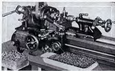
Fig. 609.—Forming and Cutting Off Duplicate Parts from Bar Stock
