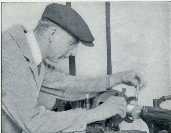
Fig. 439.—Using a Micrometer Caliper Measuring Work in the Lathe
