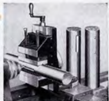
Fig. 591.—End-Milling a Keyway in a Shaft
