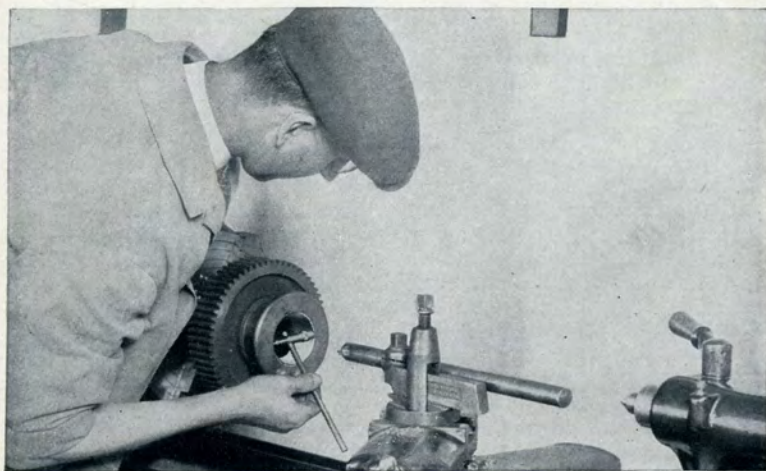
Fig. 440.—Using an Internal Micrometer Caliper Measuring the Diameter of a Machined Hole
