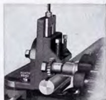
Fig. 590.—Milling a Standard Keyway
