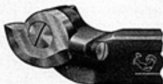
Fig. 11. Formed threading tool, solid type.
