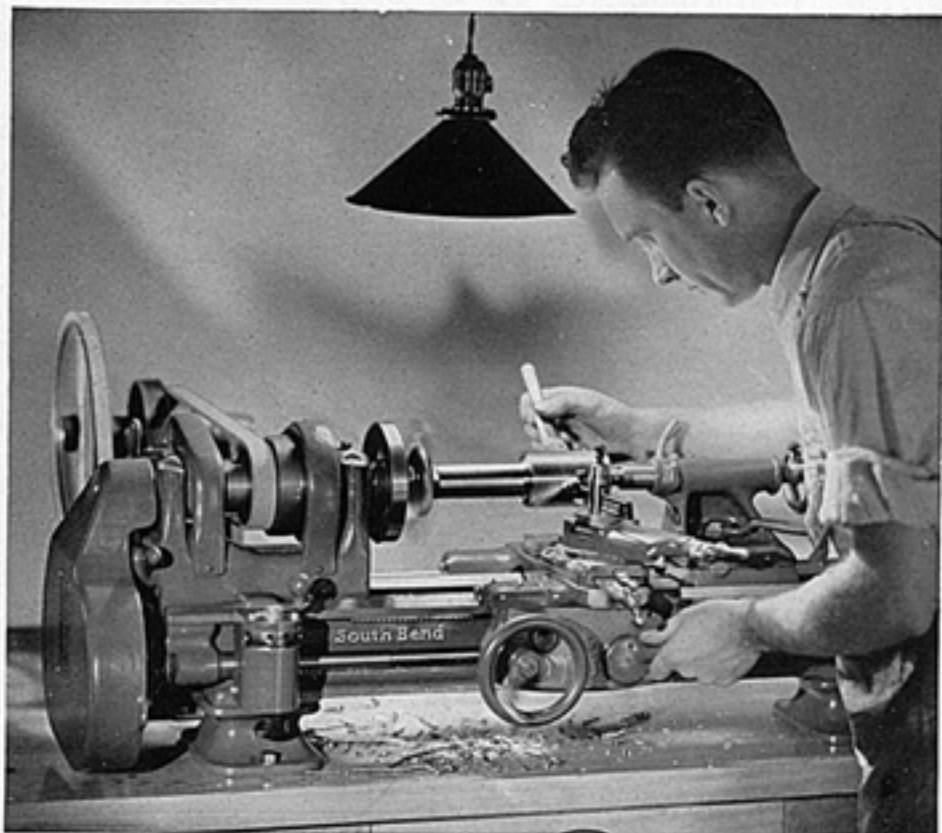
Fig. 34. Applying lard oil to work with small paint brush while cutting screw threads in a tool steel thread gage.
