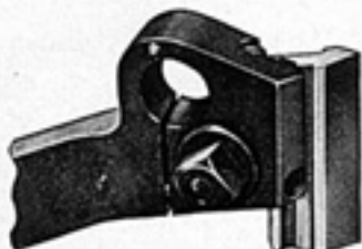
Fig. 12. Formed threading tool, spring type.
