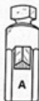
Fig. 10-A. End View of lathe tool cutter bit ground for cutting screw threads.
