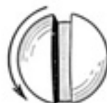
Fig. 42. A left hand screw advances when turned counter-clockwise.
