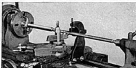
Fig. 26. Cutting a long slender screw thread, with the aid of a follower rest.
