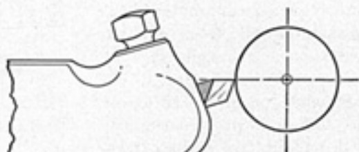
Fig. 15. Top of cutter bit should be set on center for cutting screw threads.
