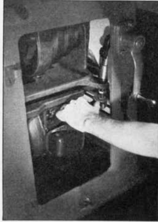
Fig. 10. Adjusting cone pulley belt tension.
