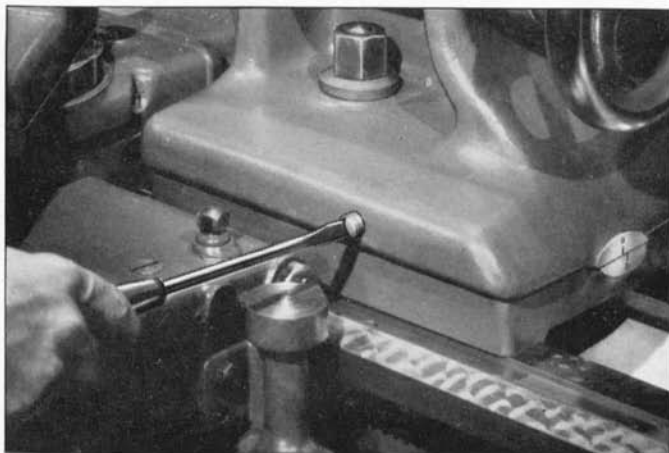
Fig. 32. Adjusting tailstock set-over screws to align centers.
