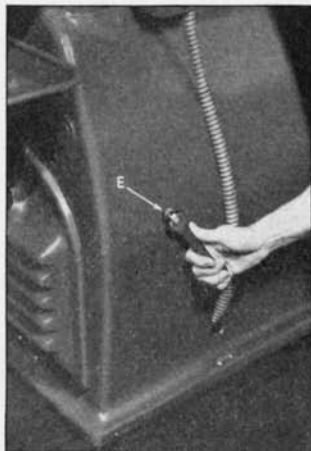
Fig. 6. If lathe is equipped with stop screw "E", it must be unscrewed before adjusting belts.
