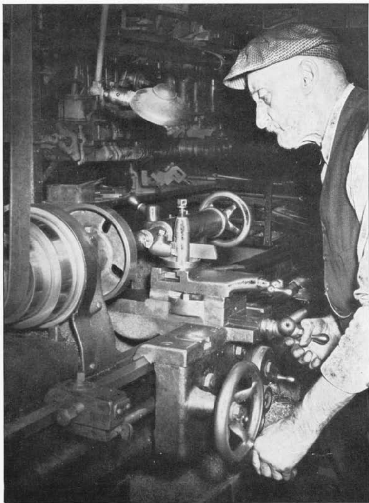
Fig. 1. Given the proper care, a good lathe will retain its accuracy indefinitely. This old South Bend lathe has been in continuous service for more than 25 years and still does precision work.
