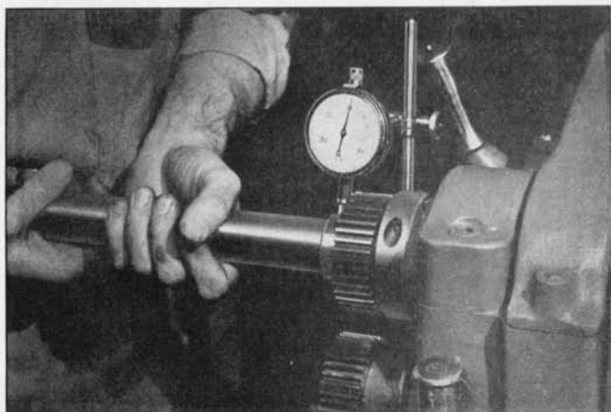
Fig. 18. Testing small spindle bearing for clearance.
