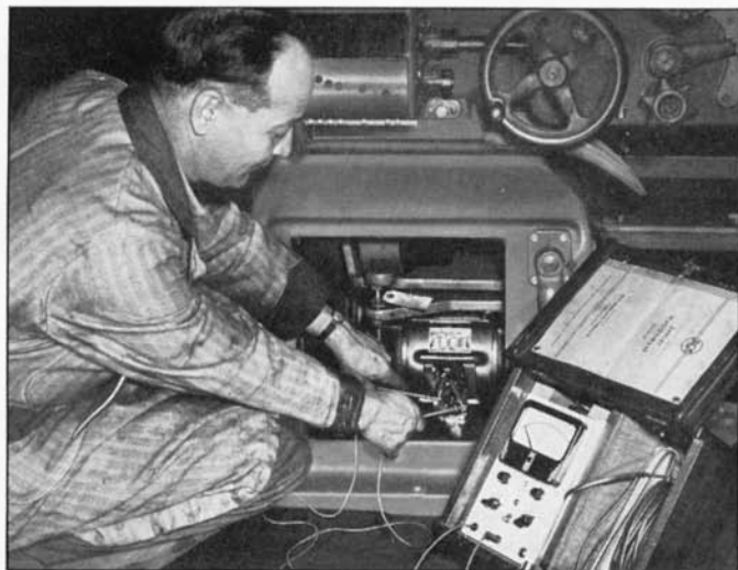
Fig. 2. Checking the line voltage at the motor.
