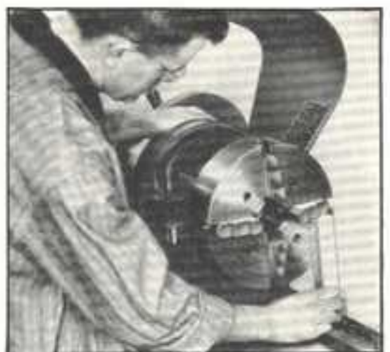
Fig. 156. Removing a Chuck from Lathe Spindle
