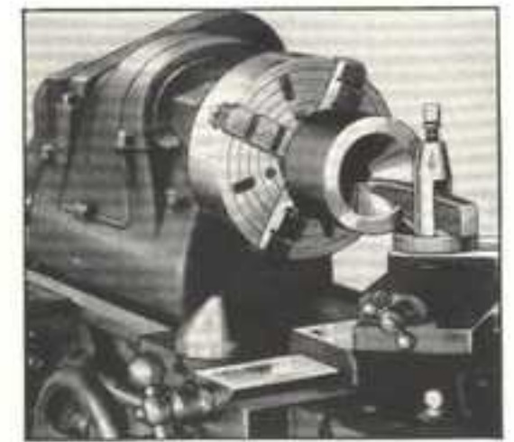
Fig. 171. Machining a Conical Punch and Die with Compound Rest
