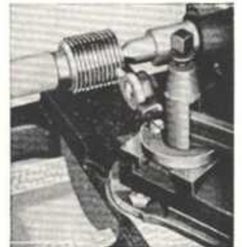
Fig. 222. Cutting a Screw Thread with Compound Rest Set at 29°
