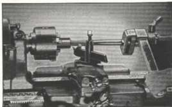
Fig. 202. Floating Reamer Driver
