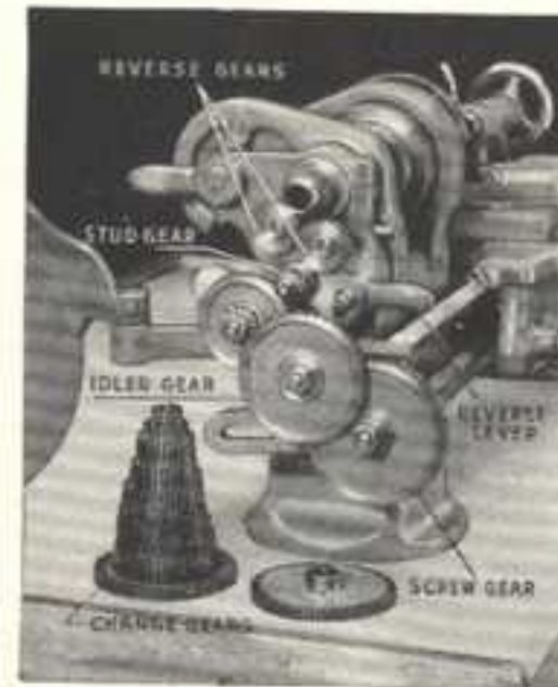
Fig. 6. End View of Standard Change Gear Lathe
