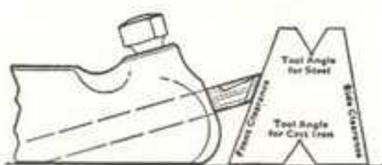
Fig. 54-B. Checking Front Clearance
