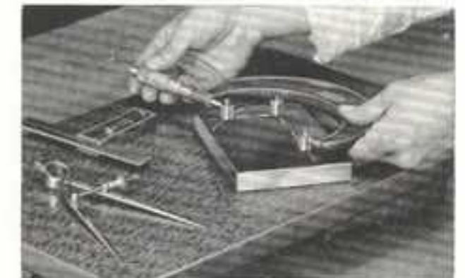
Fig. 110. Measuring Across Toolmaker's Buttons Mounted on Jig Plate
