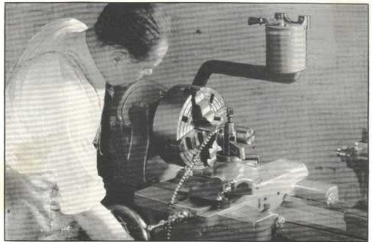
Fig. 148. Machining a Shaft in an Independent Chuck
