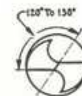
Fig. 197. Correct Point Angle
