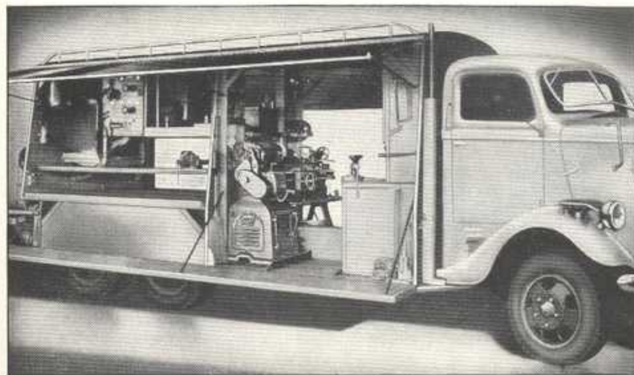
Fig. 338. A Portable Machine Shop Built in a Large Truck
