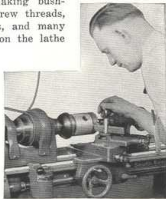
Fig. 329. Turning a Semi-Machined Piston to Size in a 9-in. Lathe
