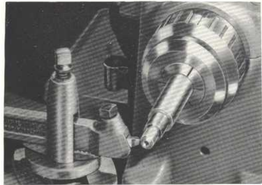
Fig. 161. Machining a Part Held in a Draw-in Collet Chuck
