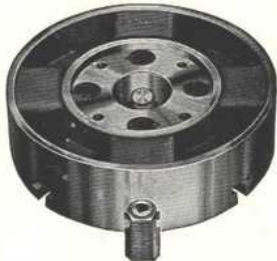
Fig. 347. Rear View of the Lathe Chuck
