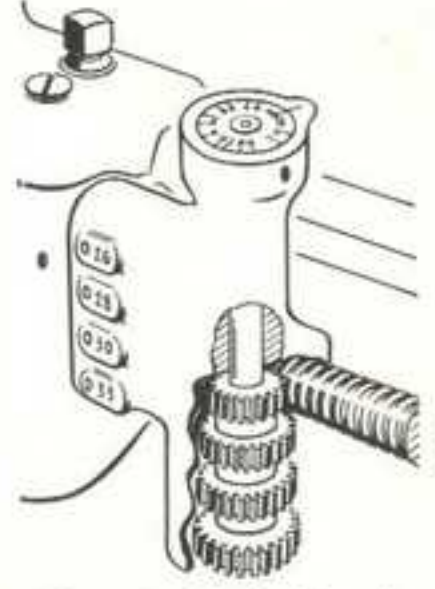
Fig. 254. Metric Thread Dial Indicator
