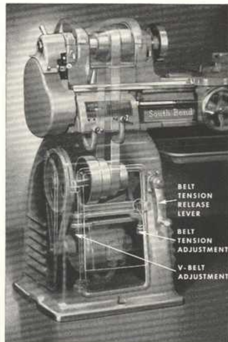
Fig. 14. Phantom View of Underneath Belt Motor Drive
