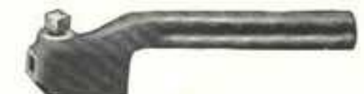
Fig. 41-A Holder for Grinding Cutter Bits
