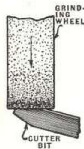
Fig. 58. Grinding Right Side of Cutter Bit
