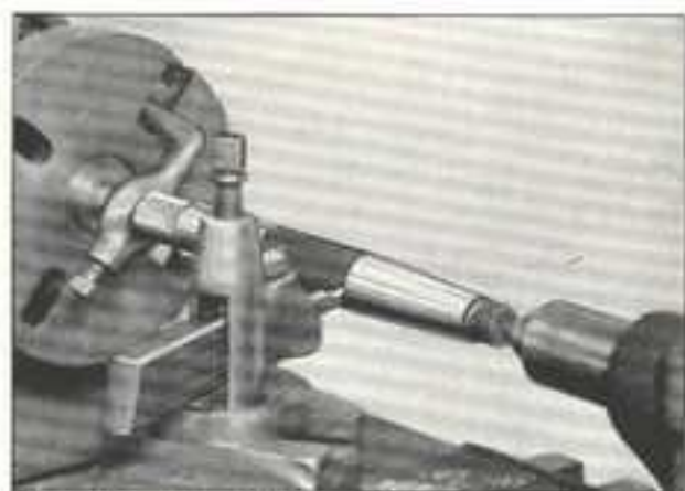
Fig. 176. Machining a Taper with the Tailstock Top Set Over
