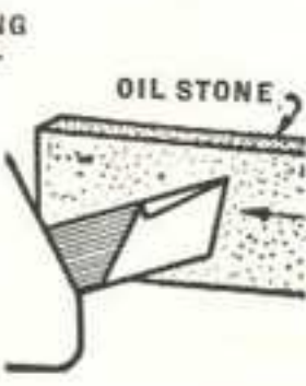
Fig. 62. Honing the Cutting Edge of Cutter Bit with an Oil Stone
