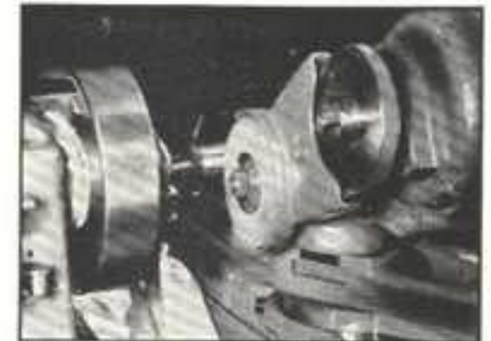
Fig. 319. Grinding a Hardened Steel Bushing
