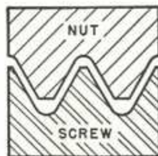
Fig. 208A. Diagram Showing International Screw Thread Form.
