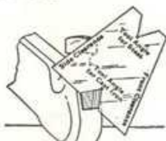
Fig. 54-C. Checking Tool Angle
