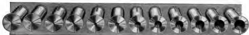
Fig. 170. A Set of Collets for Round Work \frac{1}{16} In. to \frac{3}{4} In. by 16ths
