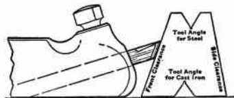
Fig. 54-B. Checking Front Clearance
