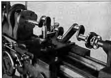
Fig. 337. Testing a Crankshaft in the Lathe
