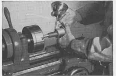
Fig. 267. Lapping the Inside of a Hardened Steel Bushing with Emery Dust and Oil
