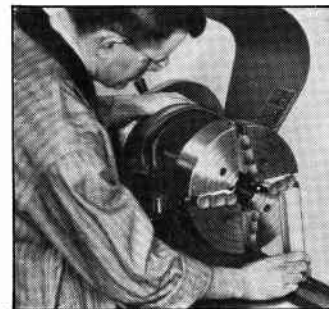
Fig. 156. Removing a Chuck from Lathe Spindle
