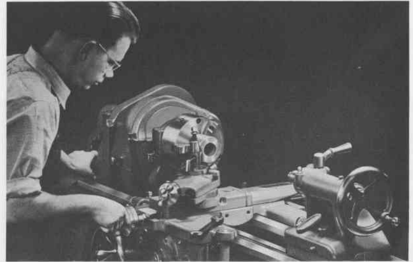
Fig. 148. Machining a Bushing in an Independent Chuck.
