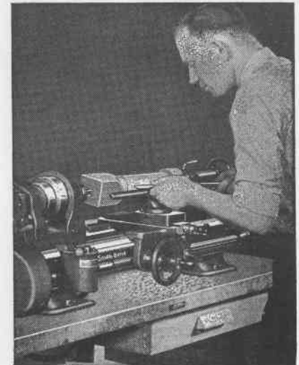
Fig. 307. Wood Turning in a Metal Working Lathe
