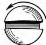
Fig. 235. A Left Hand Screw Advances When Turned Counter-clockwise
