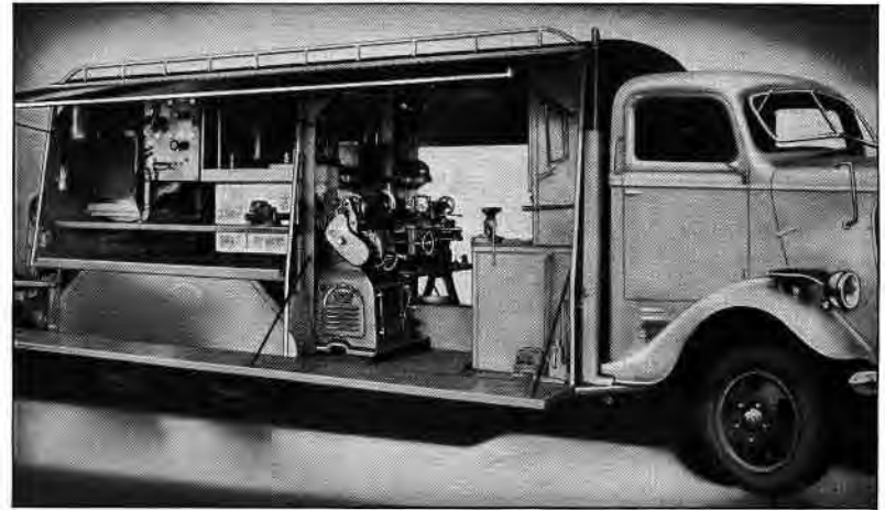
Fig. 338. A Portable Machine Shop Built in a Large Truck
