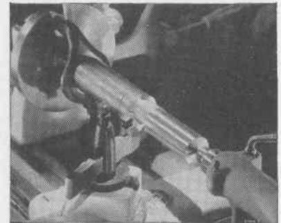
Fig. 356. Taking a Finish Turning Cut Following a Rough Turning Operation
