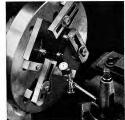
Fig. 111. Locating Work on Face Plate with Toolmaker's Button and Indicator
