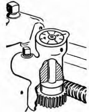
Fig. 237. Thread Dial Indicator Attached to Lathe Carriage
