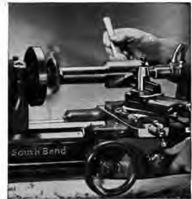
Fig. 238. Using a Small Brush to Apply Oil When Cutting Screw Threads
