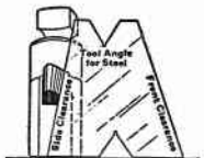
Fig. 54-A. Checking Side Clearance
