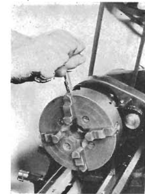
Fig. 72 Removing a Chuck
