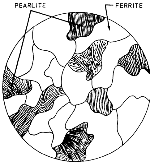
Figure 15-5.—Typical structure of low-carbon steel.
