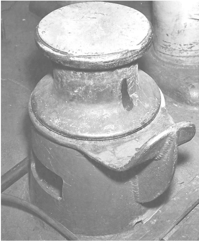
Figure 7-9.—Roller bitt saves line.
