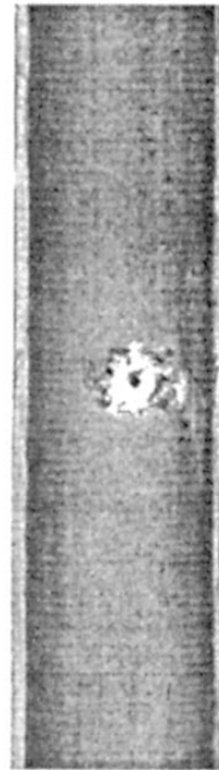
104.104 Figure 13-18.-Localized pitting (superheater tube).
