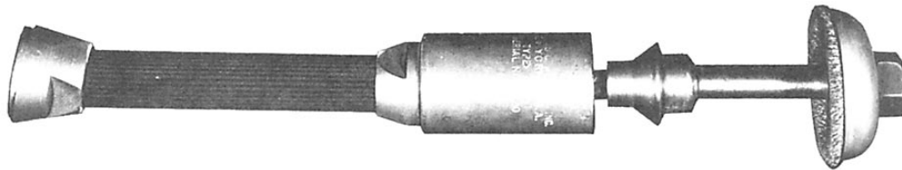
Figure 13-25.-Cup brush for cleaning handhole seating surfaces.
