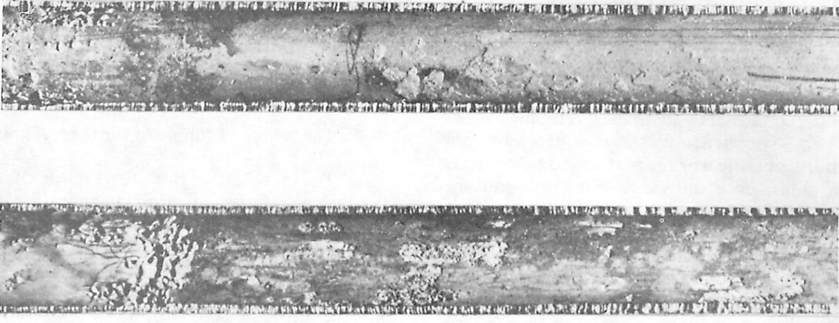
Figure 5-1.—Tubes damaged by impingement erosion.
