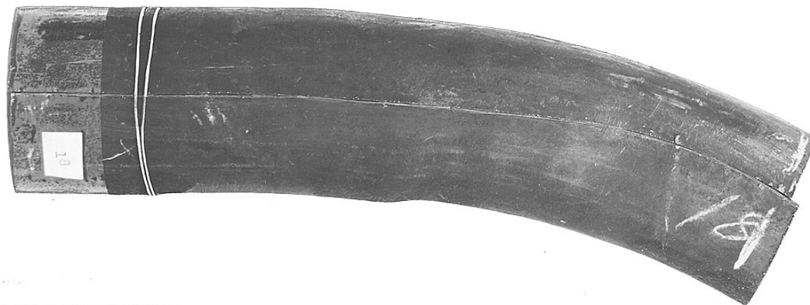
Figure 13-15.—Tube fold (fabrication defect).
