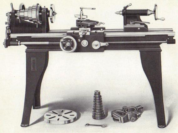
Screw Cutting Engine Lathe No. 34
