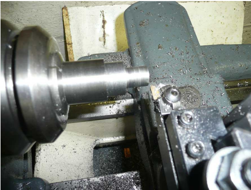
Figure 8 Turning to 0.497 Diameter.
