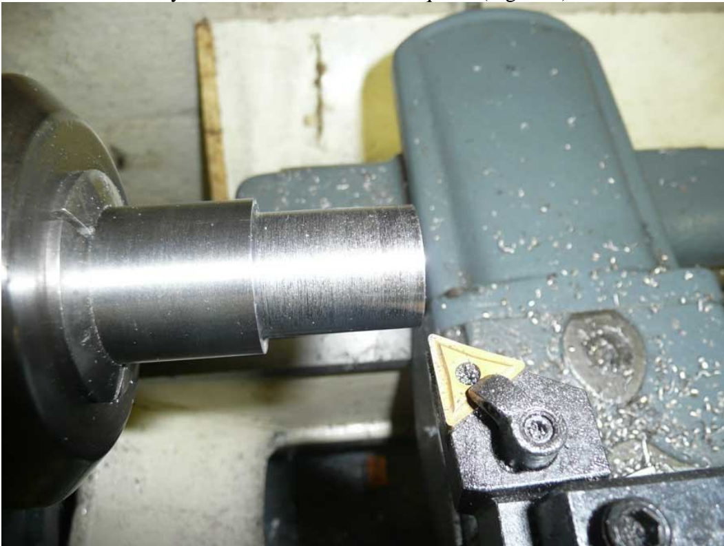
Figure 6 Starting the Inner sleeve; turning to 0.812
