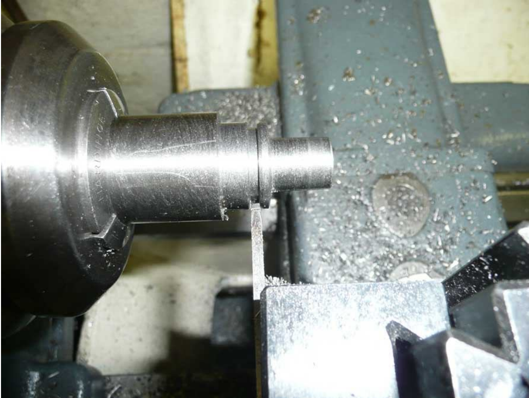
Figure 9 Parting off the New Inner Sleeve
