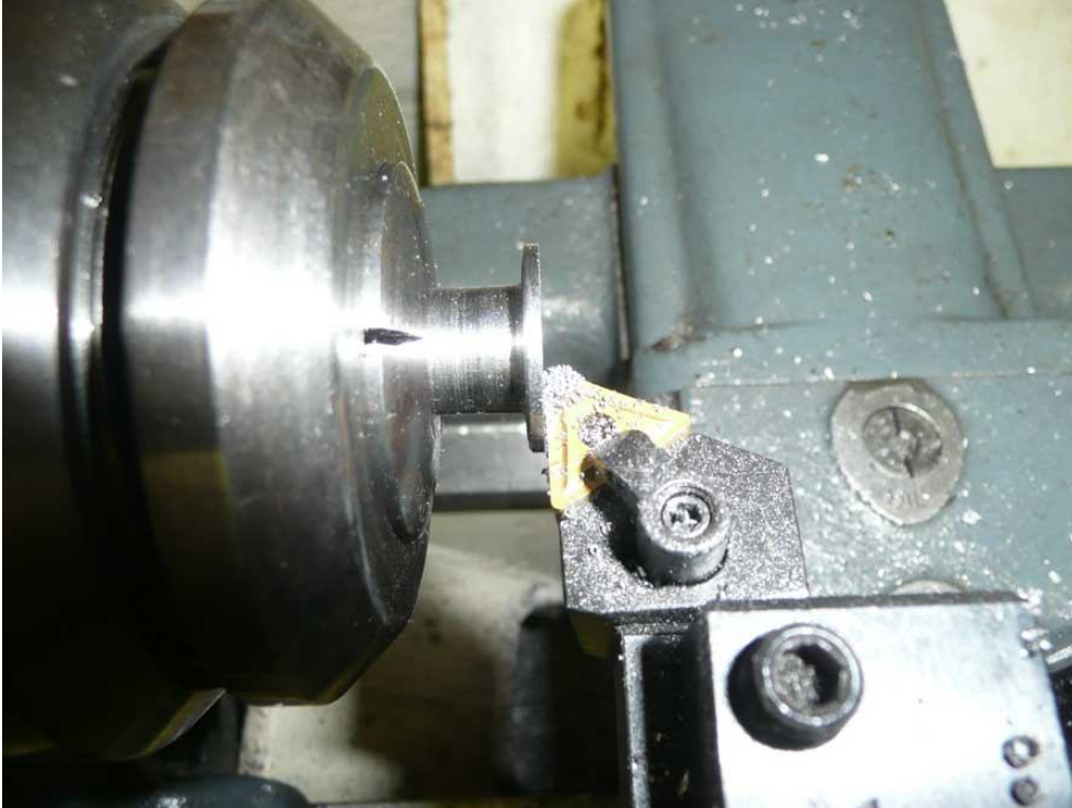
Figure 10 Trimming the Inner Sleeve Flange to 0.066"
