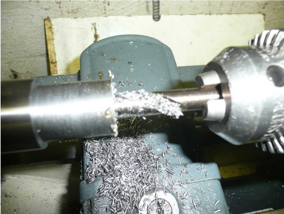
Figure 7 Drill/Ream a 0.376 hole.
